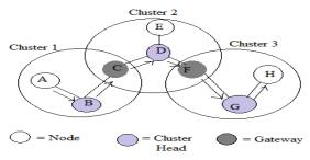
Fig. 5: Communication Diagram of CGSR via Cluster Head and Gateway.
